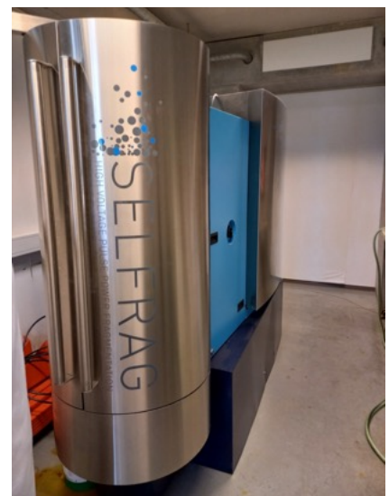
Program 2 Leader Dr Julie Hunt spent time in Belgium and Germany during the Australian winter carrying out lab work. This Selfrag equipment at the GeMME, University of Liège (Belgium), uses electric pulse fragmentation to determine if liberated scheelite (CaWO 4 ) can be produced using this size reduction methodology.
