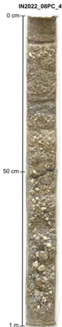
This piston core is central to PhD student Shannon Frey's work. It is an epoxy sediment peel of core IN2022_V02_08PC/4 collected from the 2022 voyage to the Kermadec arc, led by Martin Jutzeler. This core was sampled from a sediment wave on the volcanic flanks, thought to be deposited by subaqueous eruption-fed density currents travelling under supercritical flow conditions.
