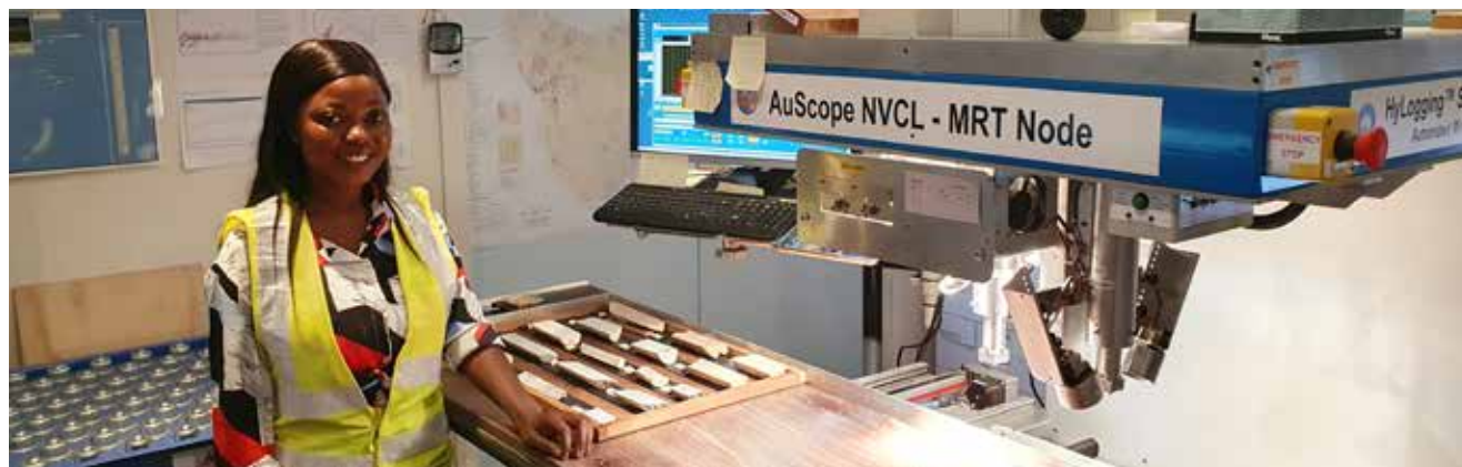
PhD student Alfredtina Appiah stands next to the Mineral Resources Tasmania Hylogger. Alfredtina uses the Hylogger to gain valuable mineralogical information about the types of carbonate and gangue silicate minerals found in Prospect Ridge ore. Pieces of drillcore she selected for this analysis are shown to her left.
