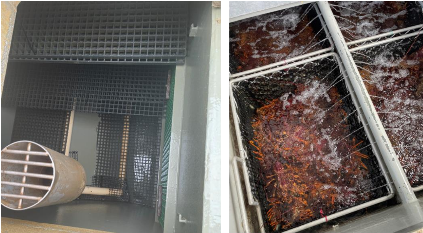
Figure 6. Good examples of two pump boat tanks. The tank on the left has a ring main water delivery loop on the base and overflow at the surface to ensure flow distribution past the lobsters before leaving the tank. The tank is subdivided into differing sections to better distribute lobsters within the tank and to provide tactile substrate for them to hold. The tank on the right uses substrate-lined baskets to distribute the lobsters through the water column and provide substrate to hold. This tank also provides water inflow which is sprayed on the surface, aiding oxygenation. However, it is noted that surface delivery of water should not be the sole source of incoming water as the new water may not reach lobsters at the base of the tank, leading to pockets of poor water quality. It is also recommended that baskets have rails on the base (and preferably the sides) to reduce the likelihood of limb damage.
