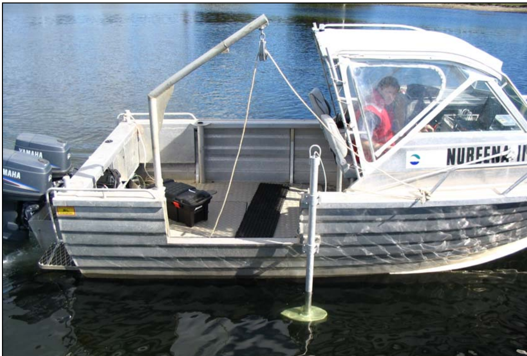
Fig. 3. Set-up of pole-mounted echosounder transducer on 5 m vessel used for inshore surveys.
