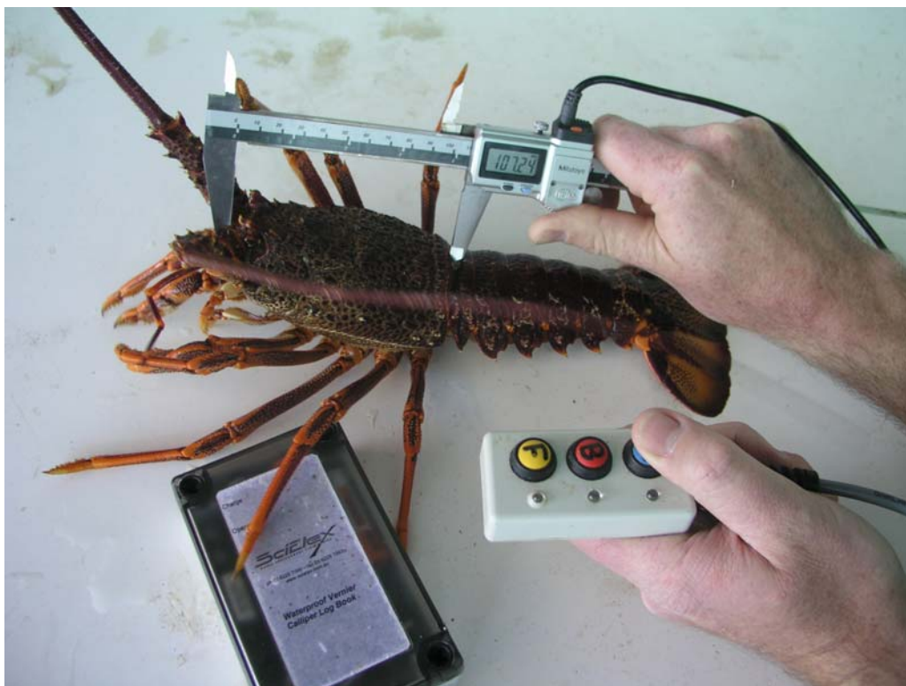
Figure 5. Measuring a lobster using an electronic data logger.
