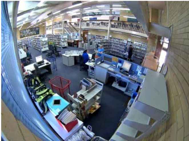
Field of view too wide, looking at walls and lights
