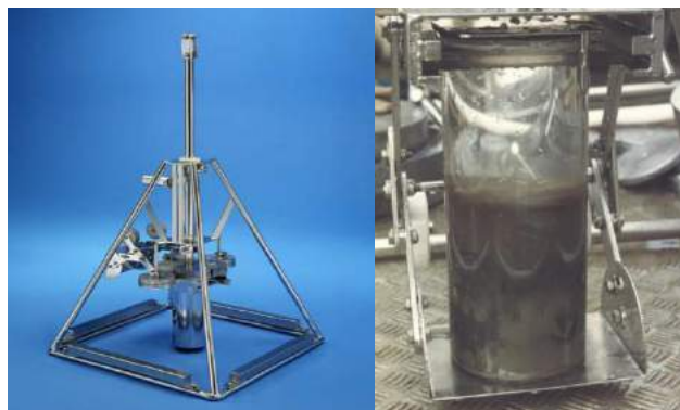
Figure 5.1-13 Haps bottom corer (left) and an undisturbed sediment core collected using a polycarbonate sample tube (right).
