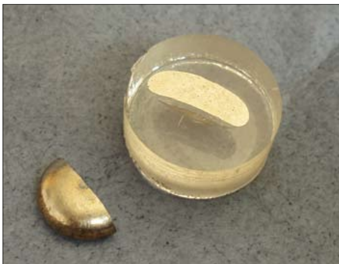
NiS standard (lower left) cut, mounted and polished (top right) ready for LA-ICPMS analysis. Project P5.F1.
