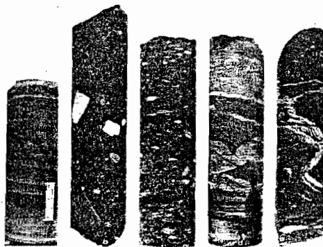
A. Core IT 28. Basal contact of Great Conglomerate with angular fragments of underlying Mowashu dolomitic shale. B. Core IT 16. Typical unsorted pebbly sandstone with clasts lacking preferred orientation. C. Core IT 28. Pebbly mudstone with elongated clasts lying flat. D. Core I-83, near Muihtra. Pull-apart structure in the Great Conglomerate. E. Core IT 28. Stump structure in the Great Conglomerate.
