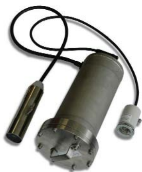
Figure 33. Digital frame grabber (left), rated to 600 m. The hard drive and battery are contained within the large metal cylinder. Lighting is supplied with a 3W LED light (equivalent light output of a 20W dichroic). Image to the right shows a frame from a shallow water trial deployment. The claws of a large male can be seen in the foreground, while a female crab outside the trap is visible in the background.
