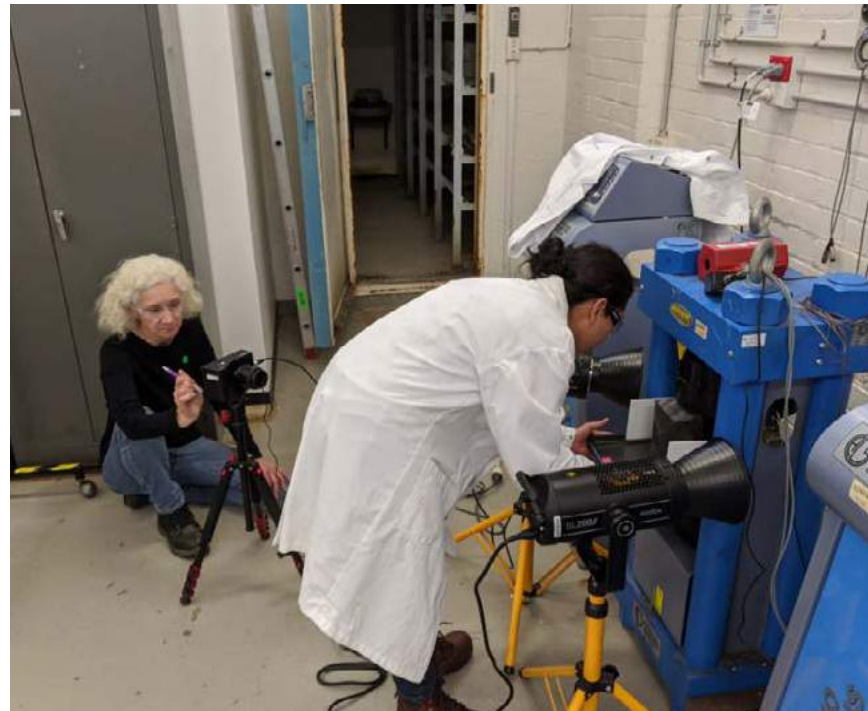
CODES Masters student Karla Morales loading samples into the crusher while Dr Julie Hunt adjusts settings on the high-speed camera, UTAS Engineering Workshop, March 2021.
