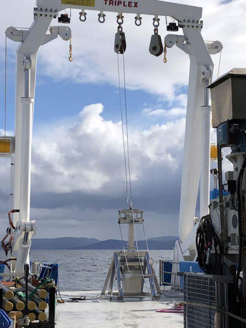
A brand-new shiny box corer on board the RV Investigator in the Derwent Estuary during a trial voyage in November/December 2021.
