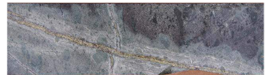
White and green mica alteration halos surrounding quartz-pyrite veins in volcaniclastic breccia from the Resolution porphyry Cu-Mo deposit, Arizona. The Amira P1202 project investigated variations in white mica compositions around Resolution to test its potential for exploration vectoring.
