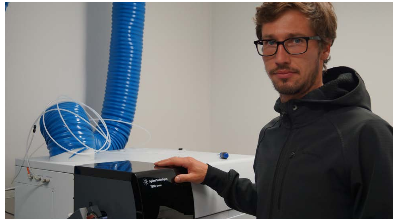
Dr Ivan Belousov is involved with the 'Development of the fast-throughput sample cell for laser ablation application' project in the TMVC Underpinning Technologies area. Here he is pictured with an Agilent mass spectrometer used for LA-ICP-MS analyses.
