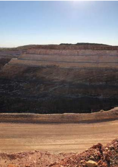
Osborne open pit (looking east). The Cu-Au mineralisation at Osborne is buried under approximately 30 m of flat-lying Mesozoic cover rocks (tan-white, from surface to third bench). The magnetite ironstones (white lines) run downwards at a ~30-degree angle from right to left across the photo. Drs Jeff Steadman and Jonathan Cloutier studied the ore host magnetite ironstones as part of the ‘Mineral geochemistry vectoring’ project, including new U/Pb age data on apatite hosted within the ironstones.
