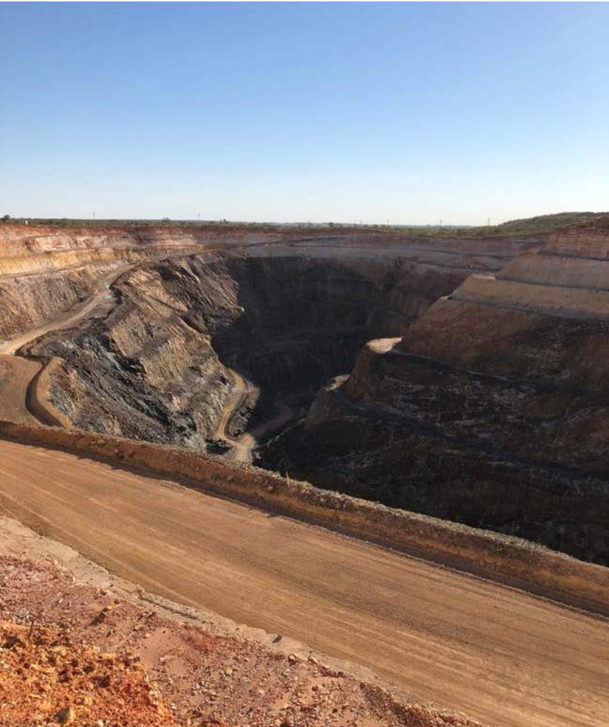
Photo (looking north) of the open pit at the Osborne IOCG deposit, Cloncurry district, Queensland, which was part of the ‘Mineral geochemistry vectoring’ project. The magnetite ironstones which host pyrite-chalcopyrite mineralisation in this deposit are visible in the sidewalls of the pit (white lines running up the walls).
