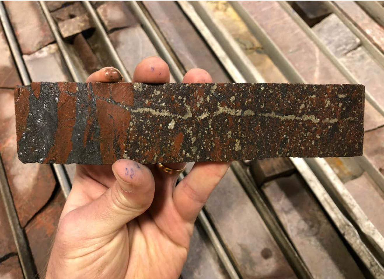
Copper-gold magnetite breccia ore in drill core from the Ernest Henry IOCG deposit, Cloncurry district, Queensland. Dr Jeff Steadman developed mineral trace element vectors at Ernest Henry as part of his work on the 'Mineral geochemistry vectoring' project. Note the zone of specular hematite on the left-hand side of the core (blue-grey colour).
