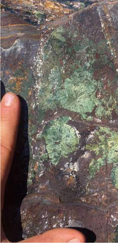
Zeb Zivkovic is undertaking a PhD at CODES on lithogeochemical fertility indicators for VHMS deposits within the 'VHMS Research – Ancient' project. Here he holds this sample of radial chlorite on Archean banded iron formation, from the Ilaara Greenstone Belt, Yilgarn, Western Australia (discovered during fieldwork in April 2021).
