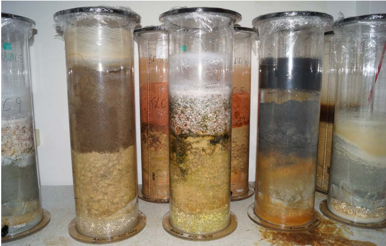
Kinetic leach test columns from Annah Moyo's PhD study, where industrial wastes were trialled as covers for mine wastes over a period of 100 weeks. Each column was subjected to wetting and heating cycles and water quality was monitored weekly to assess the effectiveness of the industrial waste covers in managing water quality.
