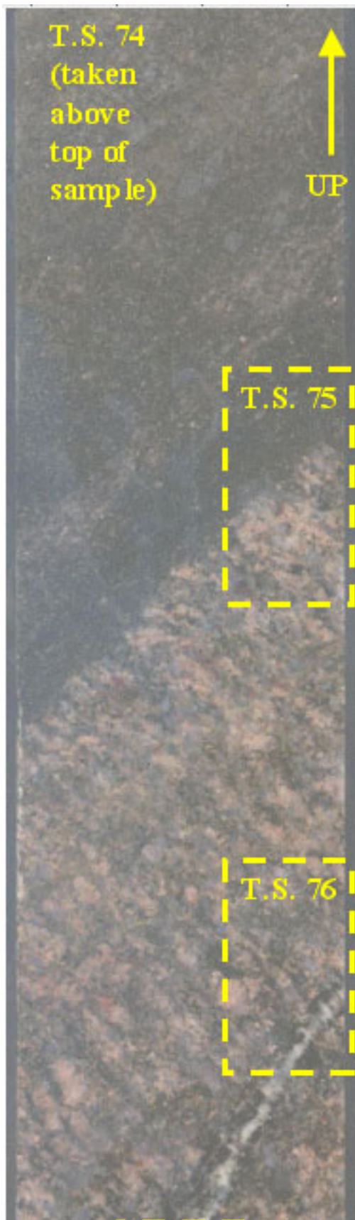
Figure 8. IT28, 5098 ft. Contact between Lower Roan quartz arenite and basement "gneiss". Note faint layering in arenite parallel to the contact and to the hematite vein, high angle "gneissic" banding in basement.
