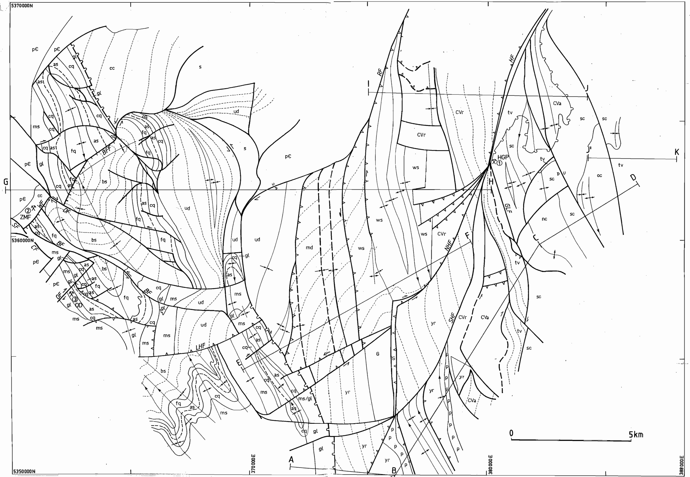
Fig. 1 Geological map of the Zeehan-Lake Selina region. Geological interpretation is based on data from this study; Blisset, 1962; Pitt, 1962; and mapping by K.D. Corbett and A.V. Brown compiled at 1:25,000 by the Geological Survey of Tasmania. ZMF= Zeehan Mineral Field, HGP = Henty Gold Prospect, OD = Oceania Pb-Zn deposit. BF= Balstrup Fault, BFF = Brickfields Fault, NHF = North Henty Fault, SHF = South Henty Fault, HF = Henty Fault, RF = Rosebery Fault.
