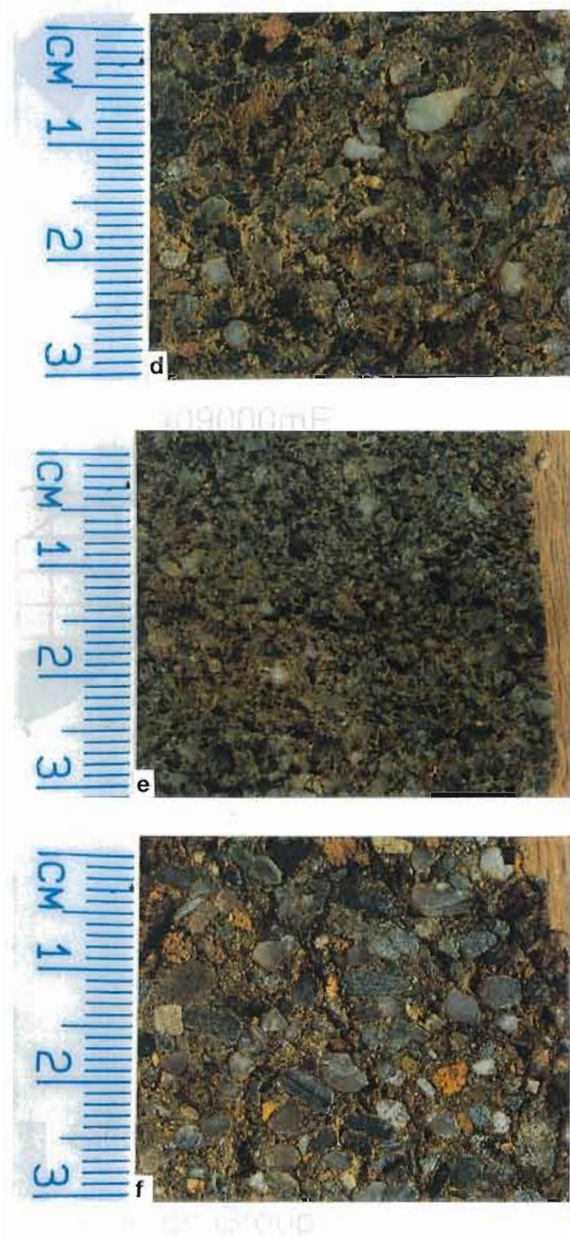
Fig. 2. Textures of coarser sediments from the Murrays Road Greywacke: (d) granule conglomerate from location B, (e) coarse sand-tone from location A, (f) granule conglomerate from the Cradle Mountain Link Road.
