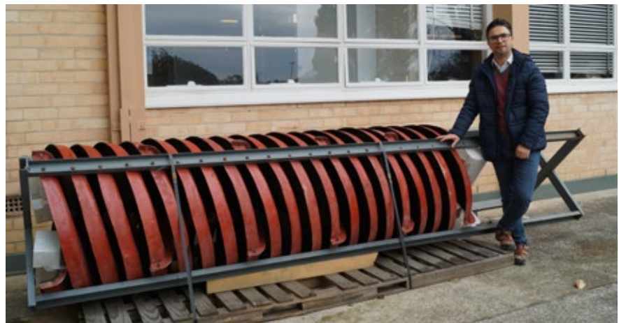
Dr Mohammad Fathi with the newly acquired spiral, set to be installed in the geology lab area at CODES. This equipment will be utilised for gravity separation-based preconcentration processes, specifically for scheelite.
